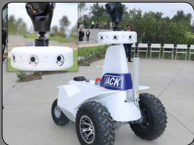
TBC-France a supplier of advanced security robotics solutions has incorporated 360 Vision Technology’s new Invictus high-performance ruggedised all-in-one PTZ camera into its advanced autonomous security robot, Jack.
