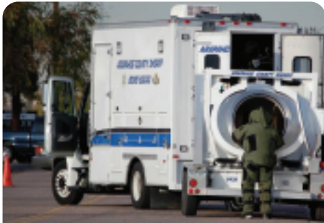
Containing bombs to effect a controlled and confined explosion is often the only way to render them safe. © NABCO
